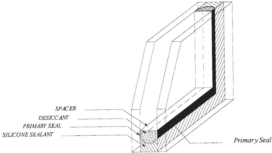
FIG. 1 Cutaway Section of IG Unit Edge Seal
